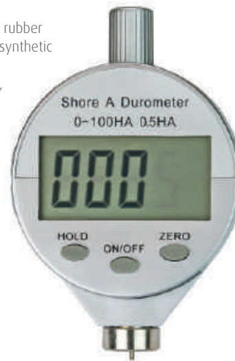
A: Flache Kegelspitze (ø 0,79mm), 35° Flat cone point (ø 0.79 mm), 35 °
